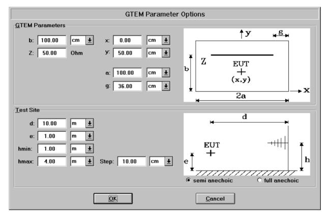
The fields **GTEM Parameters** permit to set the dimensions of the GTEM cell. The geometry of a GTEM cell is defined by a = b and g = 0.36 \* a. The values x and y indicate the middle of the test item. These values are normally x = 0.0 and y = 0.5 \* b. When changing the value b, the values for a, g and y are automatically adapted. The value Z indicates the impedance of the GTEM cell, the standard value for Z is 50 ohms.
